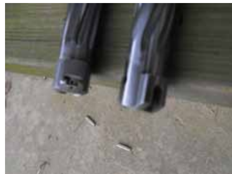
The Panda action (left) has a Winchester-type extractor, while the Saguaro features a SAKO-type
