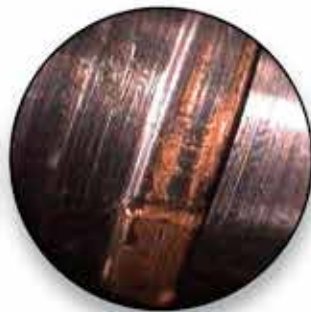
Copper, carbon & toolmarks
