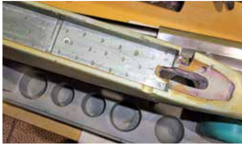
Bedding area after glued in sleeve removed.
