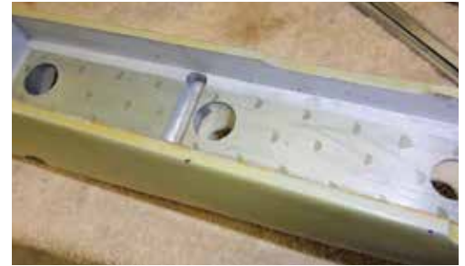
Pillar holes milled, recoil lug mortise enlarged and original bedding surface being milled away.
