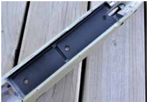
Completed bedding with edges relieved and action screw holes chamfered.
