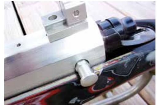
Sinclair spring loaded bolt stop and stop installed to replace the threaded screw it originally had. A recess was milled in the sleeve so the bolt release was in as far as possible.
