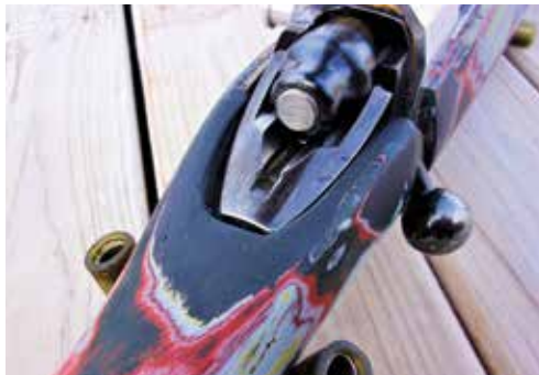
Tang area being reworked. You can also see the different colors that have been on the stock. Trigger cross pin holes have been filled and bolt handle notch has been reshaped.
