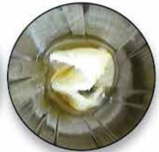
Cleaning patch in bore*
